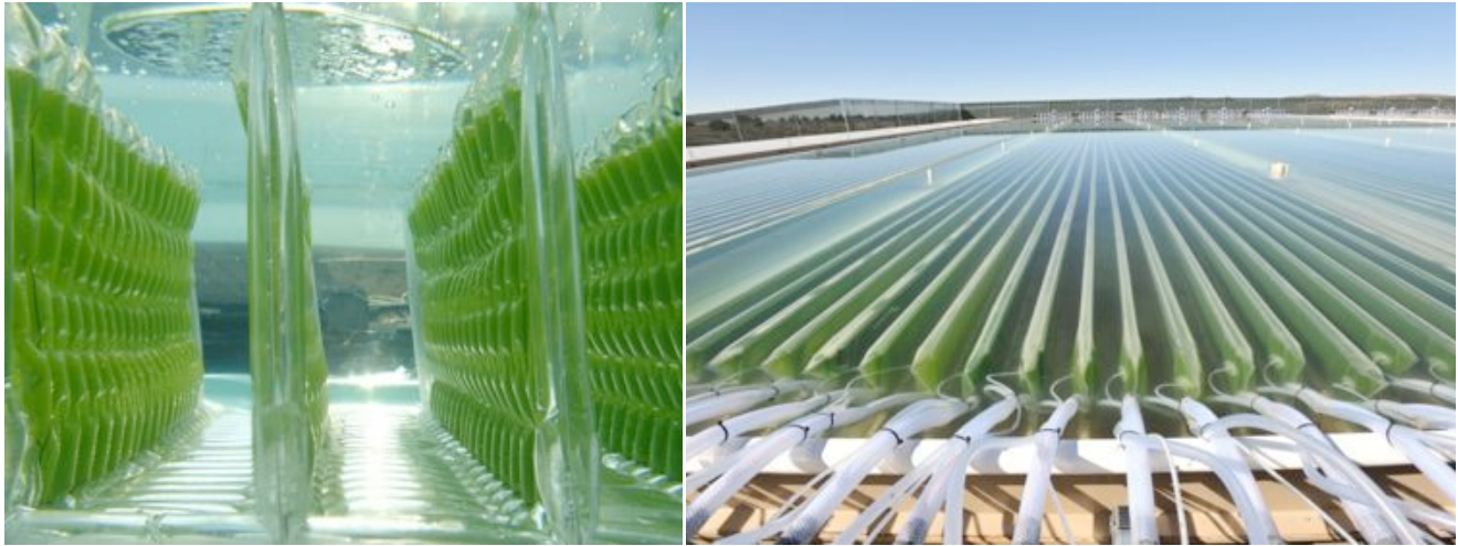
Figure 6.2 Development of low-cost, flat panel photobioreactors from (left) Proviron, Belgium, and (right) Solix Biofuels, USA. From: Wijffels & Barbosa, 2010.
