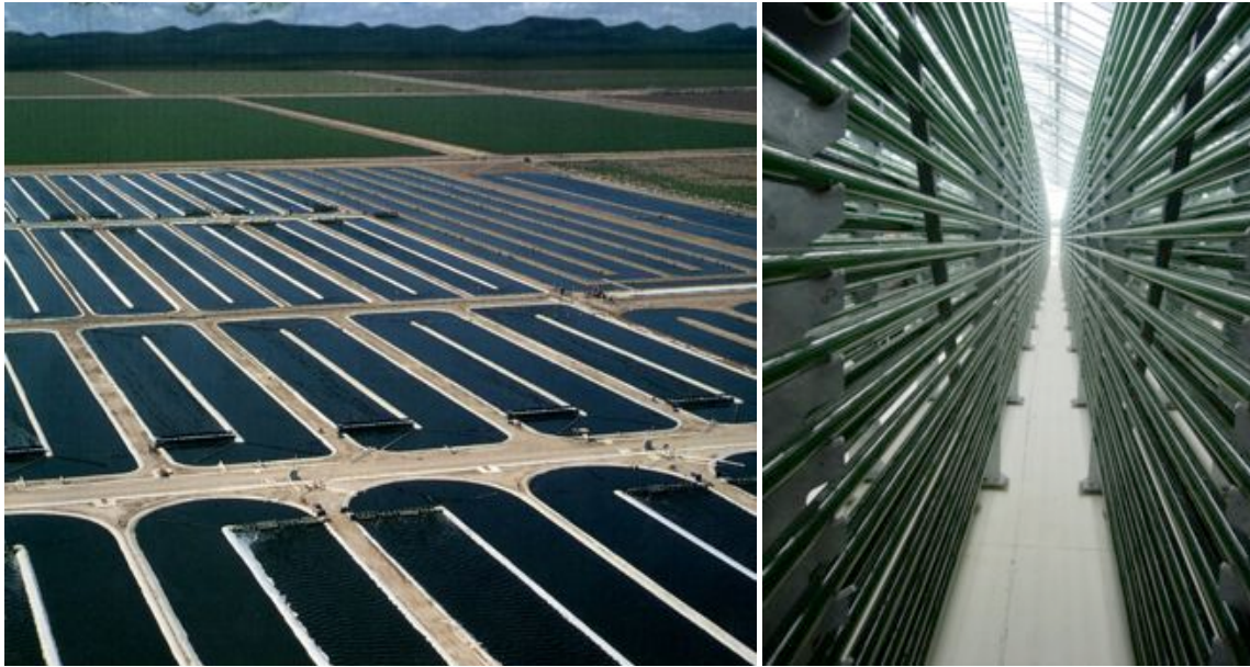
Figure 6.1 Photobioreactors for algae cultivation. Left: High Rate Algal Ponds, Earth Rise Farms, USA. Right: Tubular photobioreactor developed by IGV, Potsdam, Germany.
